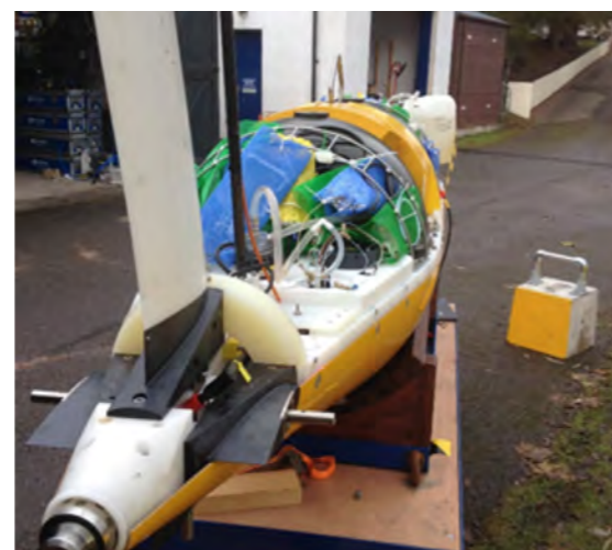
AutoSub Long Range (ALR) with total Alkalinity and pH lab on chip sensors
