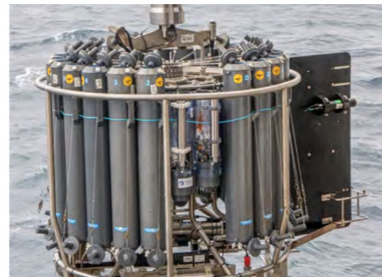
pH lab on chip sensor mounted on CTD frame during deployment at the PAP site
